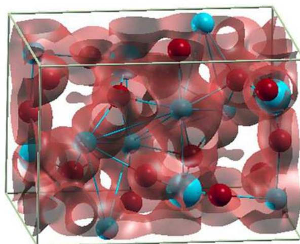
Electron density of state of LUMO in belite cement
